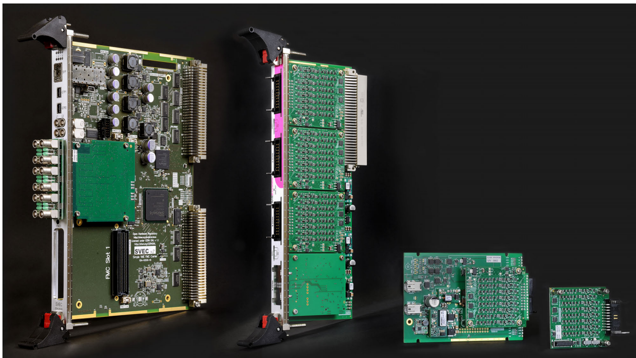
Figure 3: The different boards of the VDIO system. From left to right: small FMC board with front connectors mounted on a 6 HE SVEC VME board, RTM carrier with four rear mezzanine boards, deported IO baseboard with attached mezzanine, single rear mezzanine board.
