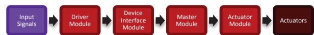
Figure 1: The BIS (red) transmits the input beam permit signals from the monitors and sensors to the actuators, which stop the beam in case of a hazard.
