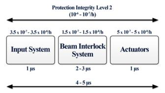
Figure 2: Shown is the PIL2 requirement and resulting tolerable failure rates allocated to different systems. The fastest reaction time and its allocation to the different systems are shown as well.
