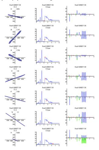
Figure 4: Transverse space 200 keV -10 MeV HB; Left: Phase space distribution X' (rad) vs X (m); Center:  $\epsilon^{N}_{X}$  in mm-mrad vs distance in m; Right: Progress of beam along Z and RF waveform
