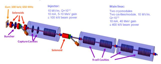
Figure 1: Schematic of the TRIUMF E Linac.
