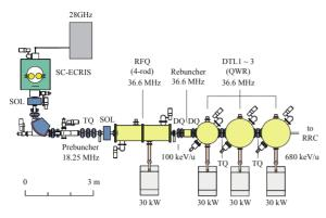
Figure 3: A plan of the new injector.
