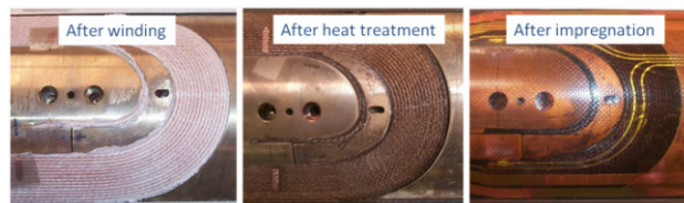
Figure 1: Nb 3 Sn coil after winding (left), after reaction (center), and after impregnation (left).
