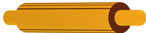
Figure 1: GdfidL model for the azimuthally symmetric beam pipe with resistive insert. The chosen length was L = 30\text{ cm} , the insert thickness a = 5\text{ mm} , the pipe radius plus the insert thickness b = 10\text{ mm} , and the electrical conductivity \sigma_c = 7.69 \cdot 10^5\text{ S/m} for Carbon Fiber Composite (CFC).
