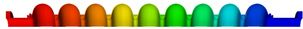
Figure 7: Lorentz force displacement of the TESLA cavity using a quarter model of the geometry.
