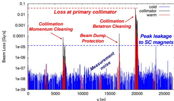
Figure 3: Beam losses throughout the LHC ring as measured during a test of the collimation system.
