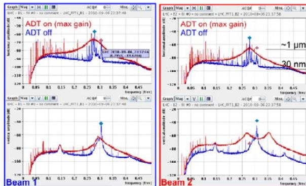
Figure 4: Comparison of tune signals with transverse damper on (red) and off (blue).
