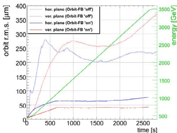
Figure 5: Comparison of orbit stability and drift with and without orbit feedback
