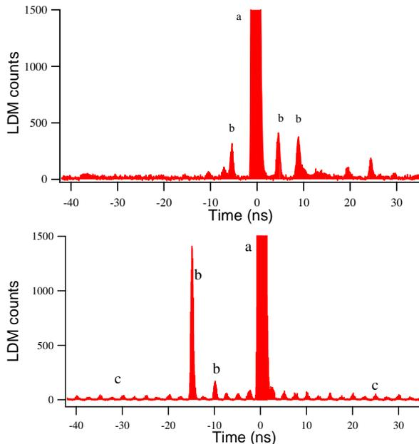
Figure 7: LDM plots for protons (above) and lead ions (below). a) main bunch with peak at  $1.3 \times 10^5$  counts, b) satellites, and c) ghost bunches.
