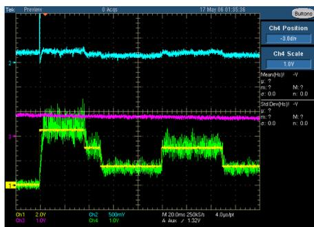
Figure 1. Time structure of extracted beam obtained by the spill control system. Spill time structure (green) can be modulated by request signal (yellow).
