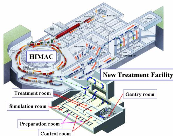
Figure 2. Layout of HIMAC and new treatment research facility. Treatments with the pencil-beam 3D rescanning have been successfully carried out at one fixed port room in the new treatment facility, since May 2011.
