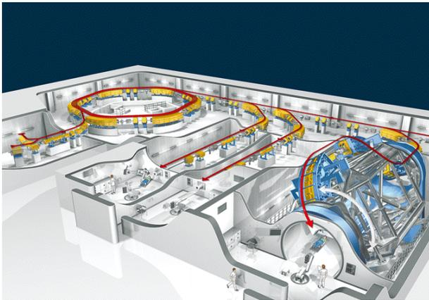
Figure 2. Layout of HIT facility. HIT facility consists of two ion sources, 7MeV/u injector, synchrotron with variable-energy operation and two horizontal fixed ports and one rotating gantry.
