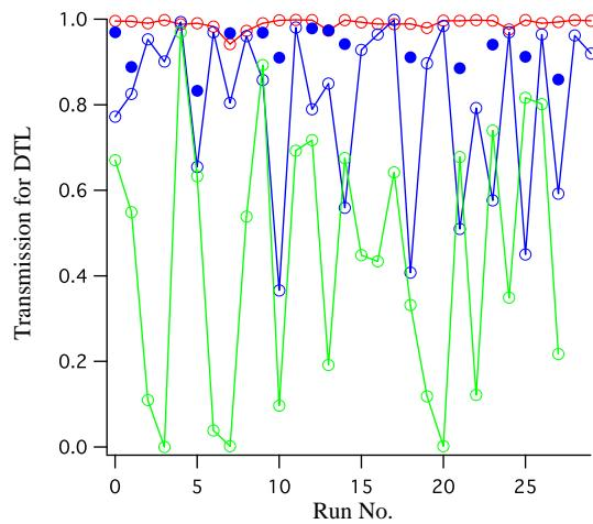
Figure 4: The simulated transmission efficiency. Red, blue, and green open circles, respectively, denote the results with the DTQ alignment error of  $\pm 0.1$  mm,  $\pm 0.2$  mm, and  $\pm 0.3$  mm. The blue filled circles show improvement of the transmission efficiency by beam steering for some cases with  $\pm 0.2$  mm DTQ misalignment.
