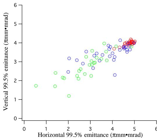
Figure 3: The simulated horizontal and vertical emittance at the DTL3 exit. Red, blue, and green circles, respectively, denote the results with the DTQ alignment error of  $\pm 0.1$  mm,  $\pm 0.2$  mm, and  $\pm 0.3$  mm.
