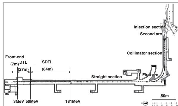
Figure 1: Scaled layout of J-PARC linac.
