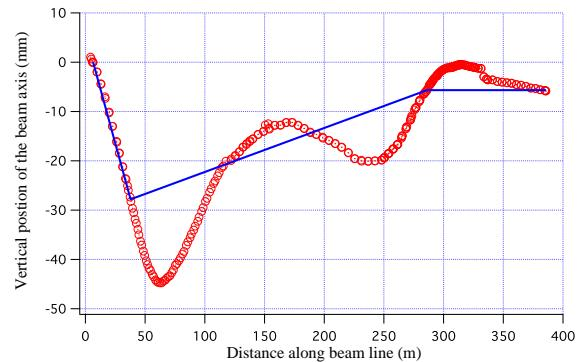
Figure 2: Elevation of linac components after the earthquake (red circles). The proposed design orbit for the realignment is also shown (blue line).
