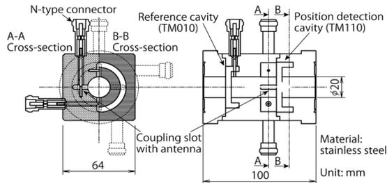
Figure 2: Drawing of the RF-BPM cavity.
