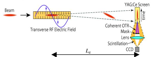
Figure 7: Bunch length measurement system using the RFDEF for a pulse width of less than 500 fs.
