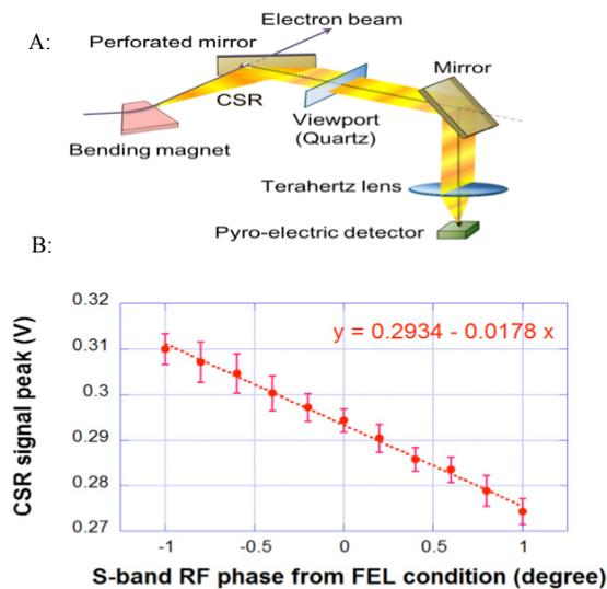
Figure 6: A. Configuration of the CSRM. B. Bunch length sensitivity of the CSRM output signal at the BC2, when the energy chirp of the bunch is changed by the rf phase in the S-band cavity.
