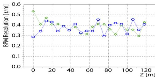
Figure 3: Position resolutions of the BPMs along the undulator beamline. The resolutions are less than 0.6  $\mu\text{m}$  (STD).
