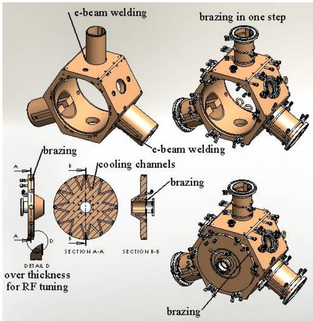
Figure 2: Main assembly steps of initial specified design.
