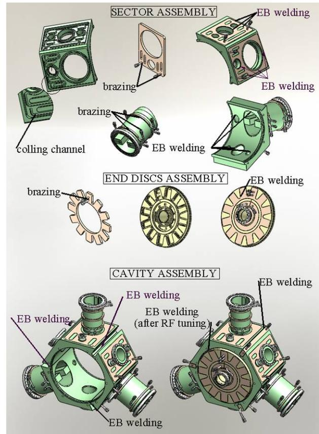
Figure 4: Main assembly steps of alternative design.
