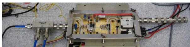
Figure 1: ELTA/SOLEIL 650 W RF module under test.
