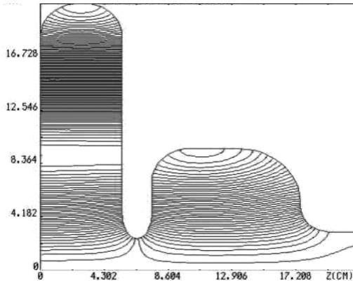
Figure 5: Electrical field lines in the gun cavity with a TM<sub>020</sub> mode in the half cell and TM<sub>010</sub> mode in the full cell. The vertical axis is the cavity radius; the horizontal axis is the cavity length.
