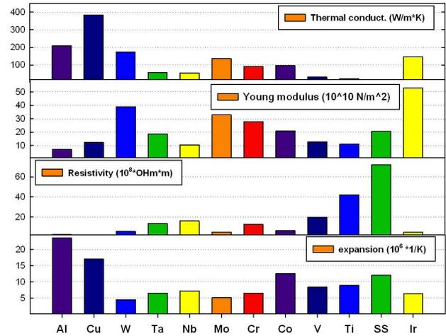
Figure 3: Some physical property of pure metals. The horizontal order ranks the metals according to the maximal gradient achieved in DC voltage test.
