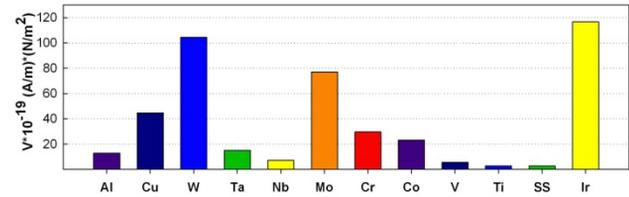
Figure 4: The ranking of metals for RF high gradient.
