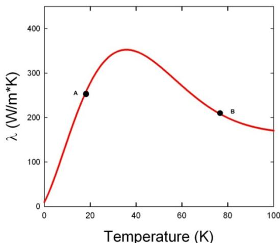
Figure 1: Thermal conductivity of molybdenum: point "A" normal operation, point "B" for cavity conditioning.
