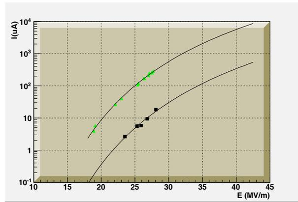
Figure 3: Dark current as a function of field, before (triangle) and after (square) treatment. The line is expected dark current based on Fowler-Nordheim theorem.
