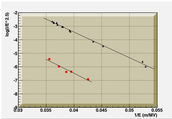
Figure 2: Fowler-Nordheim Plot of the RF processing. Field enhancement factor is extracted as 350 for the first processing (triangle) and 324 for the second processing (square).
