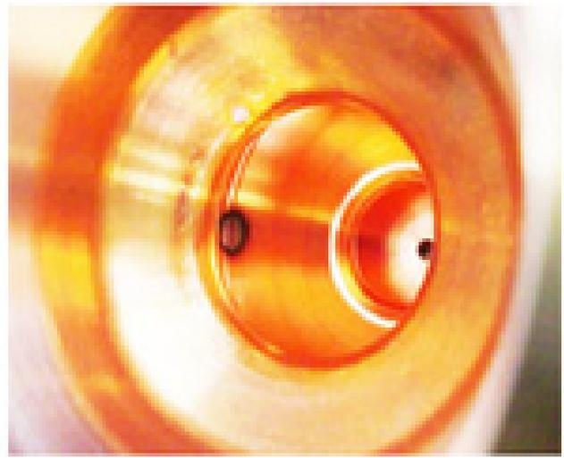
Figure 1: Picture of inner surface of the RF gun cavity after the first RF processing.
