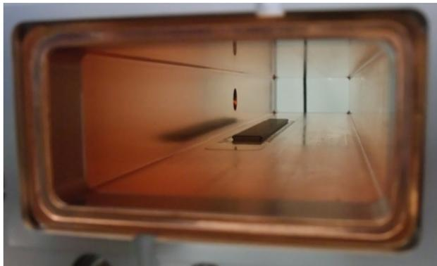
Figure 3: Ferrite located in a prototype isolator.
