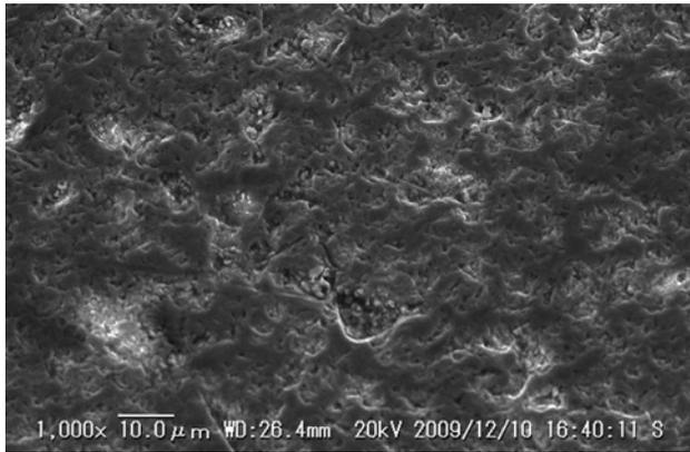
Figure 2: SEM image of a garnet-ferrite surface.
