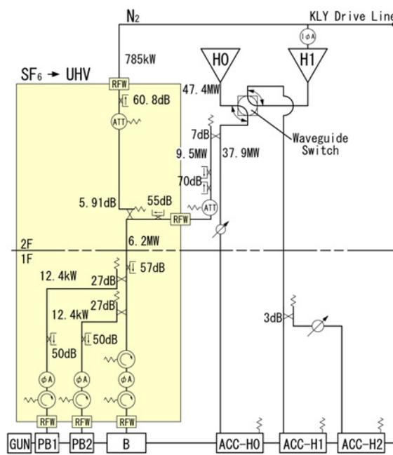
Figure 1: Waveguide system for injector section of SPring-8 linac.
