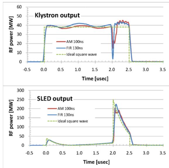
Figure 4: Typical waveform of the klystron output (upper), and the SLED output (lower), along with different amplitude modulations (see text). The green dashed line is an “ideal” waveform, assuming a square waveform with an infinity phase reversal time.
