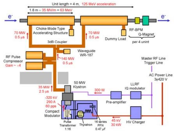
Figure 2: Configuration of C-band accelerator system.
