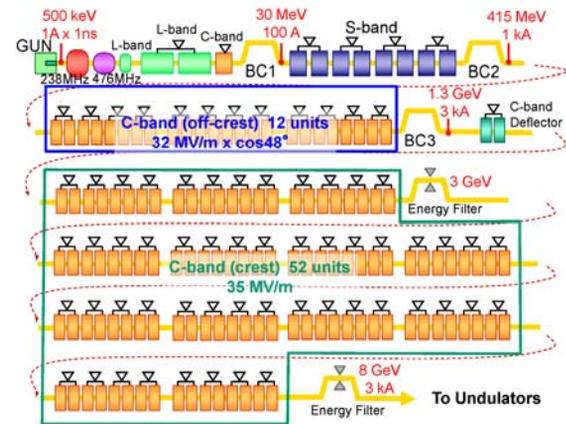
Figure 1: Configuration of the SACLA accelerator.
