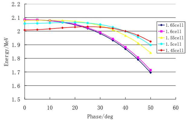
Figure 2(a): Beam energy for different half-cell length from 1.65 cell to 1.45 cell when varying injection phase.
