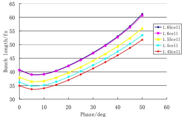
Figure 2(b): Bunch length for different half-cell length from 1.65 cell to 1.45 cell when varying injection phase.
