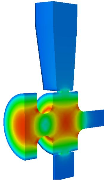
Figure 1: 3-dimensional model and pi-mode field of C-band photocathode RF gun
