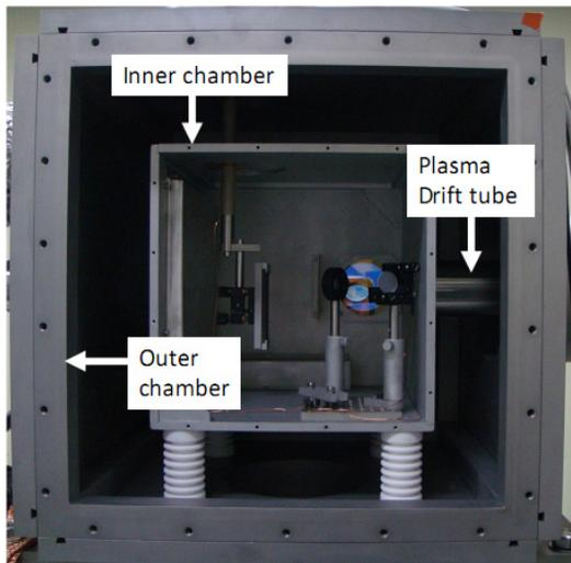
Figure 1: LIS target chamber at IMP
