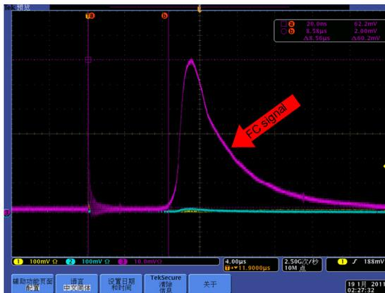
Figure 7: Non-accelerated beam signals from FFC and FCT
