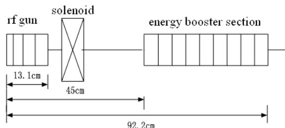
Figure 1: The THz FEL injector scheme for simulation
