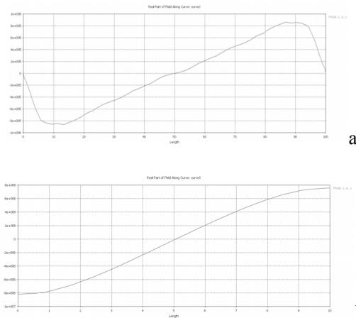
Figure 11: Resonator with vertically placed tubes distributions: electric field within drift tubes (a) – vertical axe, (b) – horizontal axis.
