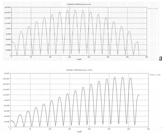
Figure 9: Distribution of E-field along of the longitudinal axe (a) –without optimization, (b) – with cutted planes
