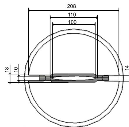
Figure 1: IH resonator with horizontally placed drift tubes. Front view.
