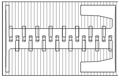
Figure 8: IH-resonator with vertically placed drift tubes and vane cutouts. Top view.
