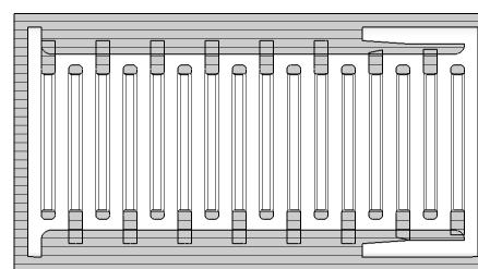
Figure 2: IH resonator with horizontally placed drift tubes and vanes cutting. Top view.
