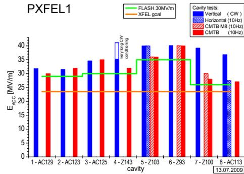
Figure 7: Cavities tests results for module PXFEL 1.
