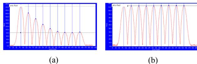
Figure 2: Field distribution of fundamental mode TM010 (a) – before and (b) – after the tuning.
