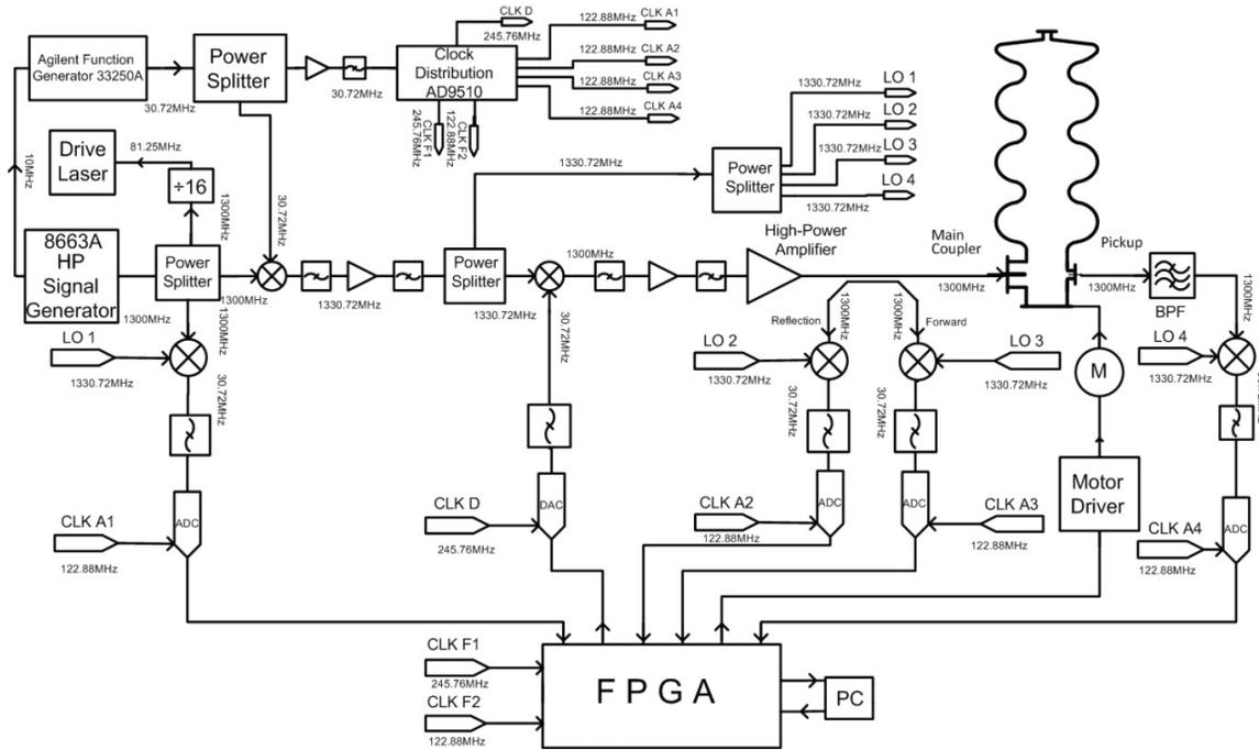
Figure 2: The schematic of the control system for PKU SRF photocathode injector.
