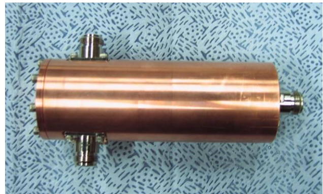
Figure 4: Fabricated split coaxial type RF combiner.
