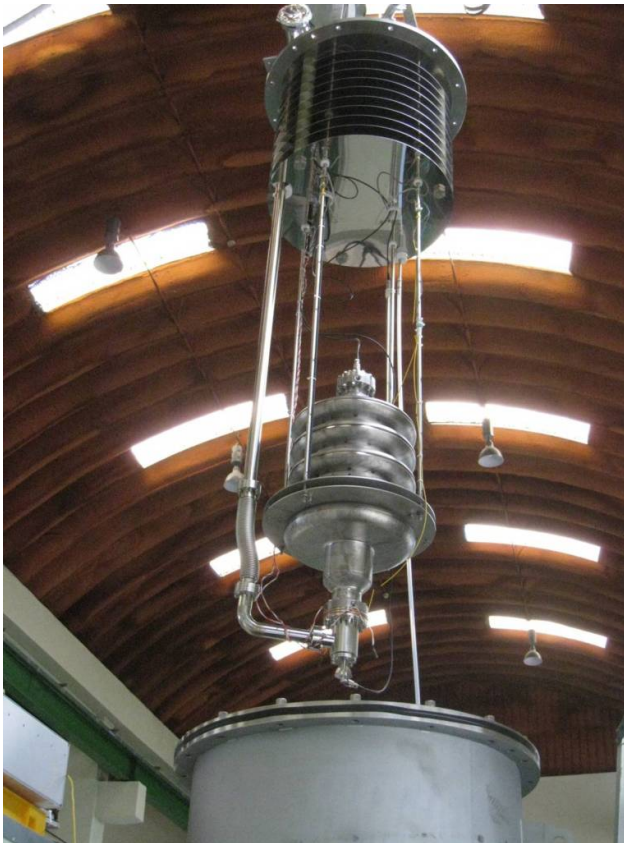
Figure 5: Insert structure with a prototype cavity.
