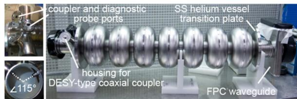
Figure 2: CEBAF 1.5 GHz upgrade type cavity (C100).
