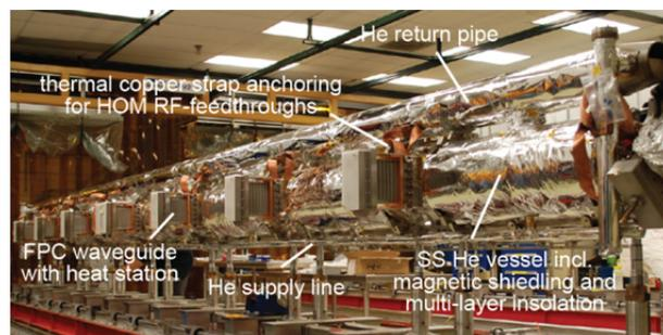
Figure 3: Cryomodule cold mass on the assembly rail.
