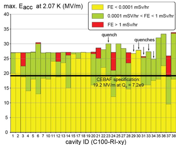
Figure 4: VTA performance of C100 cavities.
