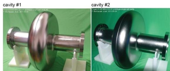
Figure 3: Medium-beta 650 MHz SRF cavities.
