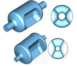
Figure 7: 750 MHz crabbing cavity (top) and 365.625 MHz deflecting cavity (bottom).
