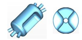
Figure 5: 499 MHz deflecting cavity (left) and the cross section (right).
