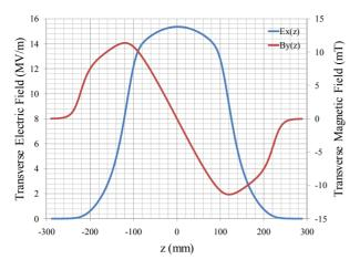
Figure 4: Transverse electric field and magnetic field along the beam line.
