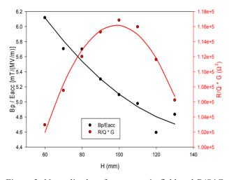
Figure 3: Normalized surface magnetic field and R/Q\*G vs. H.
