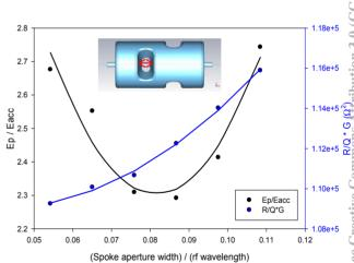
Figure 5: Normalized electric fields and R/Q\*G vs. the spoke aperture width normalized to the rf wavelength.
