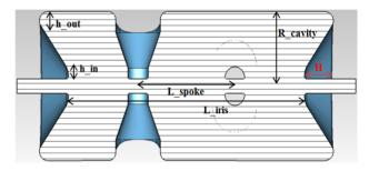
Figure 1: CST MWS cut-away view of the two-spoke 325 MHz,  $\beta_0 = 1$  cavity.
