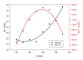
Figure 4: Normalized electric fields and R/Q\*G vs. the parameter H.
