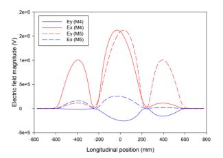
Figure 6: Transverse electric field profiles for the first degenerate pair of deflecting modes (M4 and M5).
