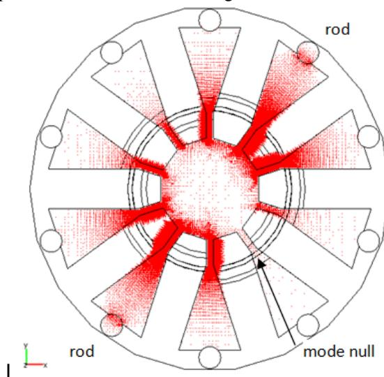
Figure 1: Next nearest mode locked in place by the ferrite/garnet rods. (The other circles in the back of the cavities are unused with vacuum characteristics in this Comsol model).
