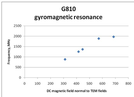
Figure 7: The gyromagnetic resonance of the YAG material as a function of the DC magnetic field in the coax test fixture.
