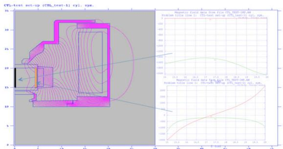
Figure 4: Modified test configuration, Poisson run and magnetic field of the main magnet, here shielded near the ferrite.
