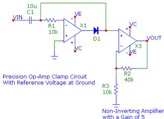
Figure 5: Two stage amplifier. First stage takes the input from -1V to 1V and shifts it to the range of 0V to 2V. The final stages amplifies it to the range of zero to ten volts
