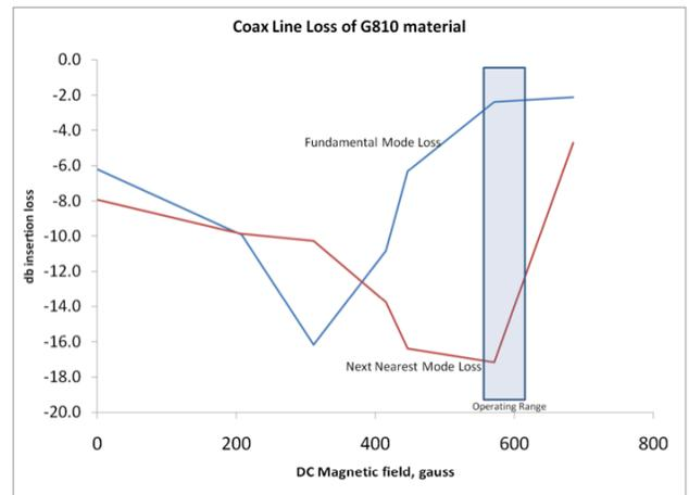
Figure 8: The loss at the fundamental frequency of the magnetron, and at the next nearest mode. The optimum level for operation is around 600 Gauss in the garnet.
