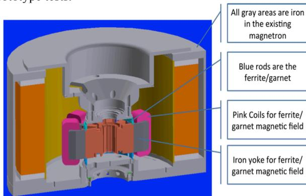
Figure 2: Cross section of magnetron tube with control magnet coils and ferrite rods
