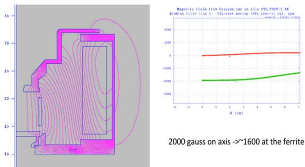
Figure 3: Present test configuration, Poisson run and magnetic field of the main magnet at the center of magnetron cavity.
