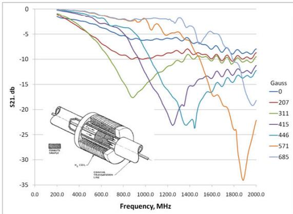
Figure 6: Test results for G810 YAG material from Trans-Tech. S21(db) in a coax line with coaxial magnetic field as a function of frequency and magnetic field.
