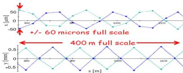
Figure 1: Horizontal ( $x$ , top) and vertical ( $y$ , bottom) difference orbit measurements in a RHIC arc.
