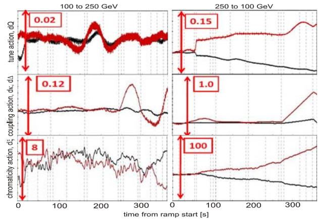
Figure 9: Action of the tune (top), coupling (middle) and chromaticity (bottom) feedback loops in the yellow ring.
