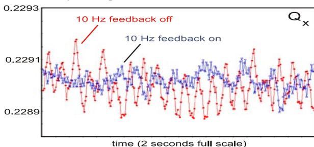
Figure 3: Measured horizontal tunes during the energy ramp with (blue) and without (red) 10 Hz orbit feedback.
