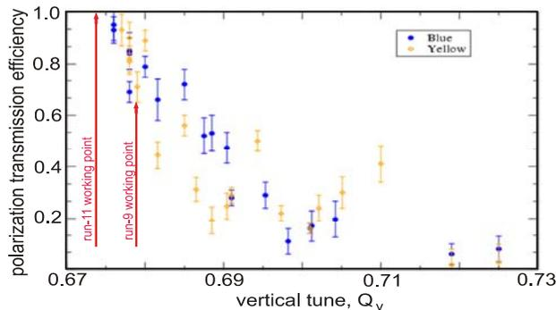
Figure 5: Polarization transfer efficiencies in the blue and yellow rings versus vertical tune setting during the 100 to 250 GeV portion of the energy ramp.
