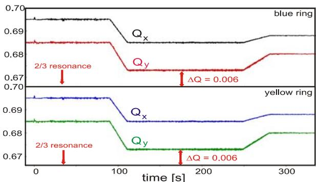
Figure 6: Tunes in RHIC during the energy ramp.
