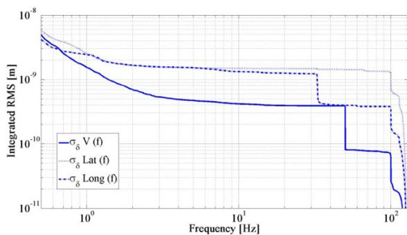
Figure 4: Calculated r.m.s. increase due to water flow
