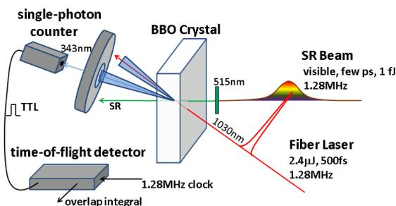
Figure 1: Cross-correlation with sum-frequency geometry.
