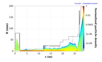
Figure 2: Beam density along the IFMIF/EVEDA prototype accelerator. Simulation performed with 10<sup>7</sup> particles.
