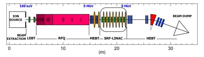
Figure 1: Scheme of the IFMIF-EVEDA prototype accelerator.
