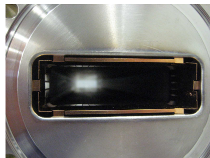
Figure 4: The fingers installed in injection kicker outlets.
