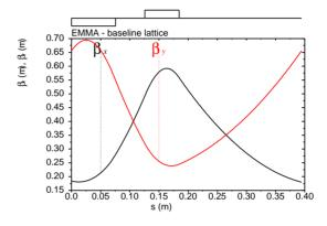
Figure 1: Beta functions for a single EMMA cell for the baseline model.
