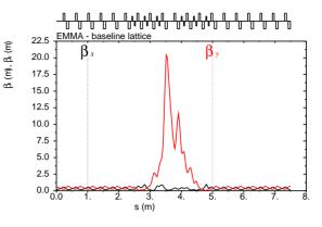
Figure 9: Beta functions with sextupoles used to match dispersion to zero in an EMMA straight.
