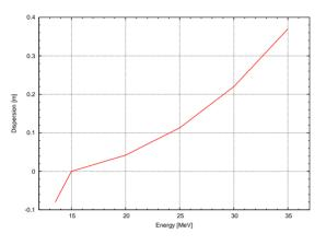
Figure 7: Dispersion versus energy in the dispersion-free straight.
