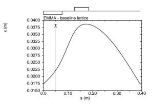
Figure 2: Orbit for a single EMMA cell for the baseline model.
