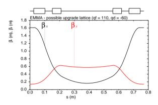
Figure 3: Beta functions when matching dispersion to zero in an EMMA straight at 15 MeV.
