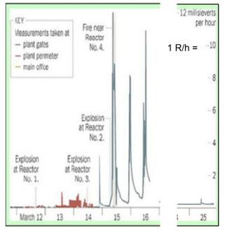
Figure 1: Radiation levels at the gates of the Fukushima power plant following the March 11 earthquake and tsunami. Twenty minutes at the peak on March 15 would correspond to the average yearly dose from natural radiation in the USA.
