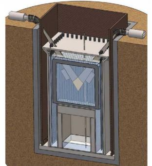
Figure 2: Conceptual design of the ADNA Green Energy Multiplier - Subcritical-technology, Thermal-spectrum, Accelerator-driven, Recycling molten salt reactor (GEM\*STAR) in its underground placement. The vertical dimension is about 9 m. The gray box is the graphite reflector for the core. Here, horizontal beams from two accelerators are shown at the top being bent by magnets into the core where they strike a uranium metal target shown schematically in the center of the core.
