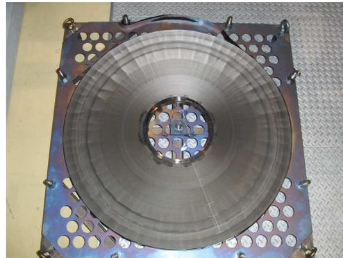
Figure 3: The first high impedance core annealed in J-PARC.
