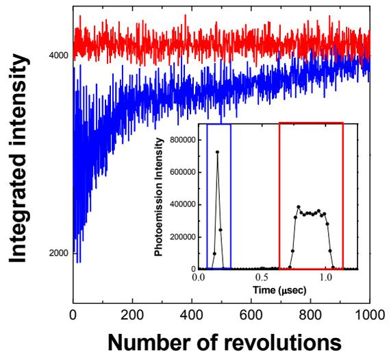
Figure 5: Integrated photon intensity recorded on the TEMPO photoelectron spectroscope for isolated bunch (blue) and multi-bunch (red).
