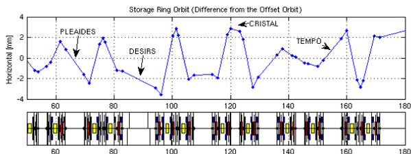
Figure 1: Closed orbit followed by the single bunch with four source-points for an orbit deviation of 2.8 mm in the undulator of CRISTAL beamline.
