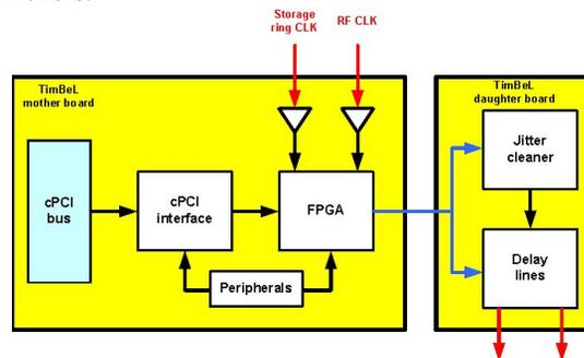
Figure 3: TIMBEL board's architecture.
