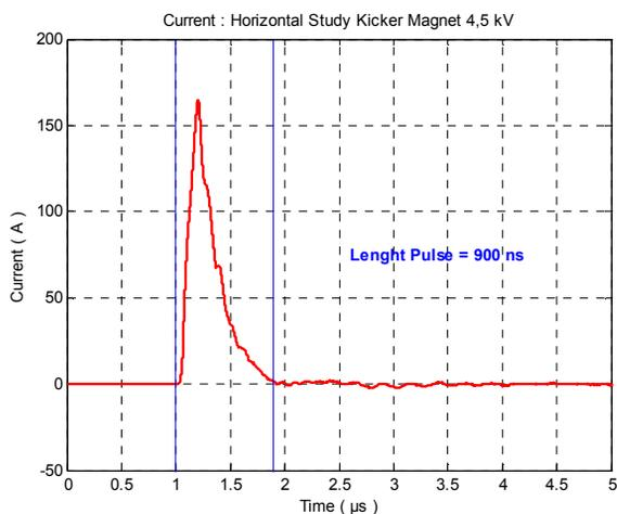
Figure 2: Horizontal time response of the horizontal fast kicker for suiting PSB requirements.
