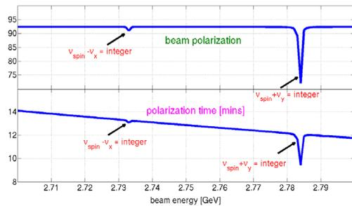
Figure 1: Beam polarization and polarization time simulated using SLIM for different beam energies on SOLEIL ring. The resonances between spin tunes ( $\nu_{\text{spin}}$ ) and betatron tunes (horizontal tune  $\nu_x$ , vertical tune  $\nu_y$ ) partially depolarize the beam.
