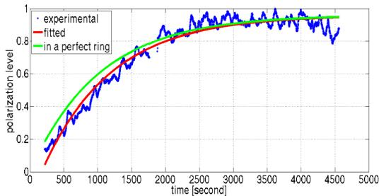
Figure 3: Polarization build up process on SOLEIL storage ring. The measured polarization is fitted using Eq.(1), then compared with the polarization on an ideal storage ring.
