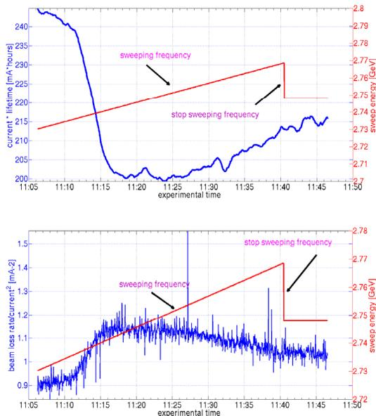
Figure 4: Upper). Normalized lifetime and down) normalized loss rate show one spin depolarization over 35 minutes. The beam energy corresponding to the sweep frequency is shown by the right y-axis.
