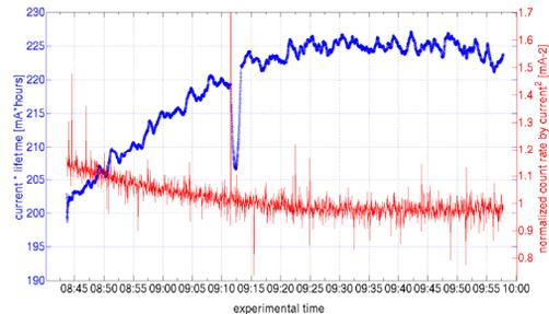
Figure 2: Beam lifetime normalized by current and beam loss rate normalized by current square. The sudden decrease of the lifetime and the sudden increase of the beam loss around 09:12 are due to the beam micro loss.
