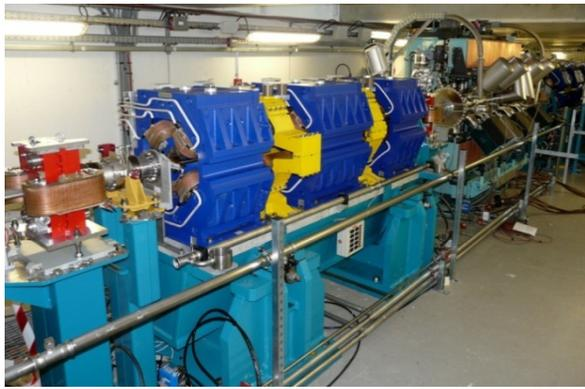
Figure 2: A part of the SDL13 straight section. That shows one magnet of the chicane (in red), one of the two additional BPMs on its Invar support, three quadrupoles (in blue), two sextupoles (in yellow) and the U18 cryogenic in-vacuum undulator.
