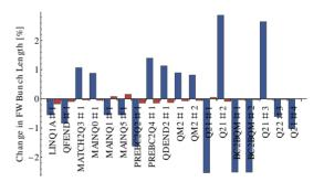
Figure 4: Change in FW bunch length from nominal on displacement in horizontal position (blue) and vertical position (green) of quadrupole by  $+10~\mu m$ . Only machines where change  $\geq 0.5\%$  shown. Unlike Fig. 3 we see that the most sensitive components are at high energy in BC2.
