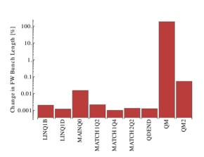
Figure 5: Change in FW bunch length on addition of +0.5% normal 12-pole field error to labelled quadrupole. Only machines where change  $\geq 0.001\%$  shown.
