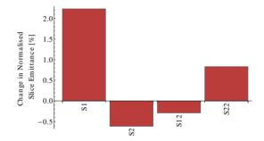
Figure 7: Change in normalised slice emittance at peak current slice from nominal on variation of sextupole field strength by +0.5%.
