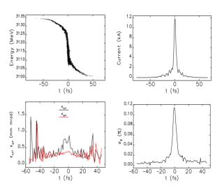
Figure 2: Baseline (SPF) final bunch properties: (1) longitudinal phase space, (2) current profile, (3) slice emittances & (4) slice energy spread.
