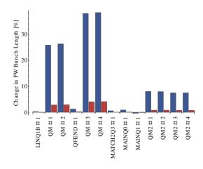
Figure 3: Change in FW bunch length from nominal on variation of quadrupole field strength by +0.5% (blue) and +0.05% (red). Only machines where change  $\geq 0.02\%$  shown. The largest 8 are within the two bunch compressors (with BC1 dominating).
