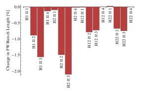
Figure 6: Change in FW bunch length under a  $10~\mu rad$  dipole roll. Each dipole is treated independently.
