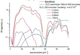
Figure 3: FTIR spectra acquired in low-alpha mode for bunch currents above the micro-bunching instability threshold (200 bunch fill pattern). Data for a black body and standard user mode are also shown.
