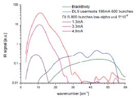
Figure 1: FTIR spectra acquired in low-alpha mode keeping the bunch current below the micro-bunching instability threshold (800 bunch fill pattern). Data for a black body and standard user mode are also shown. Beam splitter multilayer Mylar with 50 µm thickness.
