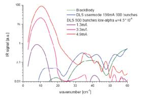
Figure 2: Same as Figure 1 with a beam splitter made of multilayer Mylar with 125 µm thickness.
