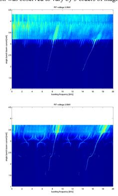
Figure 4: Spectral intensity of mm-wave emission as a function of bunch current. Data were measured using a Schottky barrier diode and a spectrum analyser. The main RF voltage was 2.0 MV and 2.5 MV (upper and lower plot respectively).
