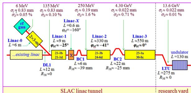
Figure 1: Layout of the LCLS machine.
