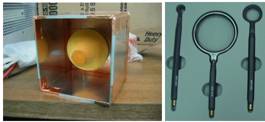
Figure 2: EMR-300 enclosed by Al 6063 boards and different sizes of Hall probes.
