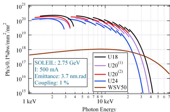
Figure 1: Spectral range covered by IVIDs of SOLEIL.
