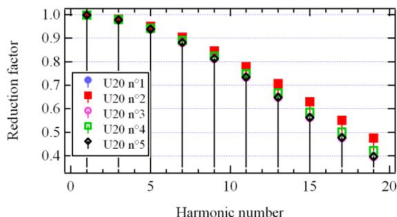
Figure 3: Reduction factor of brightness versus harmonic number.
