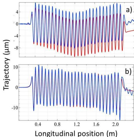
Figure 4: Measurements of the *HU60* undulator in linear horizontal mode (a) and linear vertical (b). Hall probe in red line, pulsed wire in blue. Pulse time duration fixed at  $10\text{ ms}$  with an amplitude of  $1\text{ A}$ .
