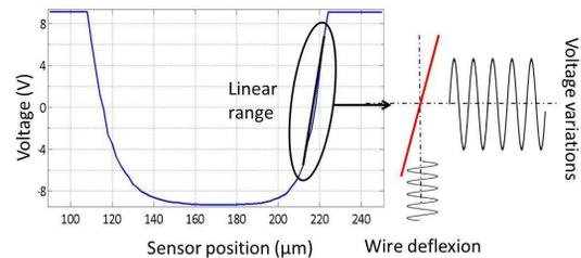
Figure 3: Voltage from a sensor according to its position while crossing the wire.
