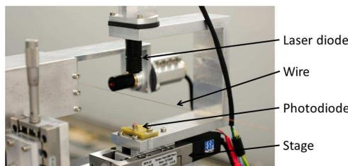
Figure 2: A detector composed of a vertical and horizontal sensor, based on a laser diode coupled with a photodiode.
