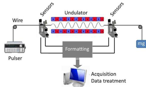
Figure 1: Set-up of the pulsed wire bench.
