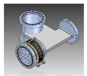
Figure 6: Schematic of RF Bellows & BPM.
