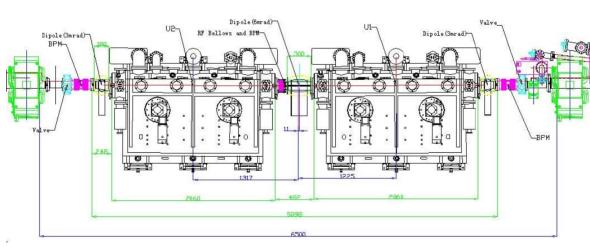
Figure 2: Layout of the components of the straight section (top view).
