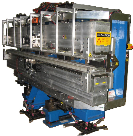
Figure 3: Elliptical Polarized Undulator (EPU46) with period length 46 mm.
