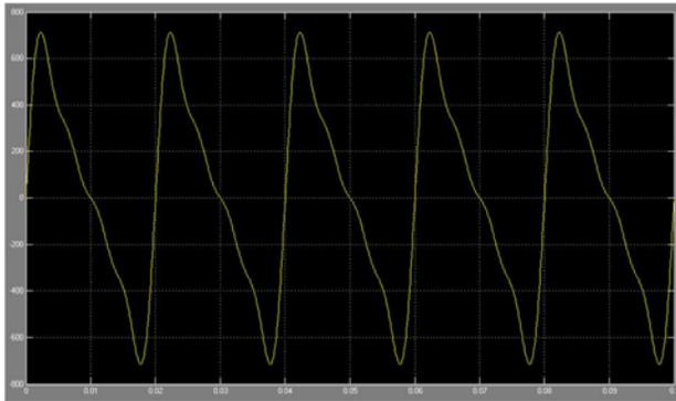
Figure 4: Wave of primary voltage.
