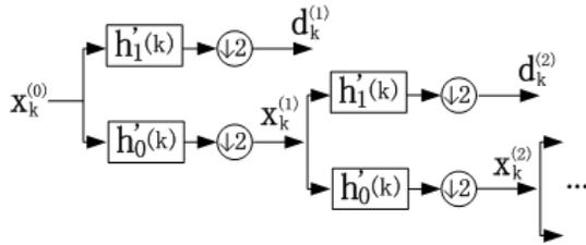
Figure 3: Process of discrete wavelet transform.
